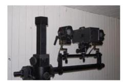
High speed camera and light sources mounted onto a studio stand, to shoot and analyse the flight characteristics of a projectile. Equipment needed : three camera holders ASNAO mounted onto two tubes ASNEU, fixed onto the horizontal beam of the studio stand with two special adaptors.
