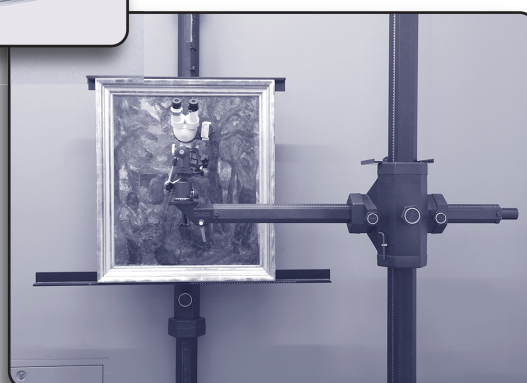
Binocular eyepiece on stand for the analysis of a work of art.
