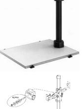
With the manual fine drive, the camera can be adjusted vertically at the desired height above the board with high precision. For a good functioning of the fine drive, the weight of the crosspiece as well as of the camera must be balanced thanks to the counterweight present in the shaft. For heavy cameras, the additional counterweight ASOBO is needed, and for light cameras, the counterweights set REPRA will equal it.
